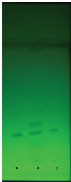
**Fig. 2.** TLC analysis. Lane A – standard vindoline with an Rf value of 0.35; lane B – ethyl acetate extract having an Rf value of 0.36; lane C – purified vindoline with an Rf value of 0.37 with the optimized mobile phase containing ethyl acetate:methanol:ammonia (6:0.3:0.1) as a solvent system.
