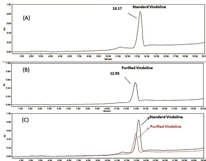
**Fig. 3.** HPLC analysis. **A** – Standard vindoline with a single peak at a retention time of 13.17 min. **B** – Bacterial purified vindoline with a single peak at a retention time of 12.93 min. **C** – Overall peak of both standard and purified vindoline.
