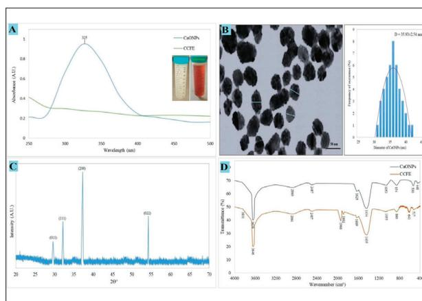
**Supplementary Fig. S2.** Characterization of CaONPs. A – UV-Vis spectrograph of CaONPs; B – TEM micrograph of CaONPs; C – XRD spectrograph of CaONPs; D – FTIR spectrograph of CaONPs.
